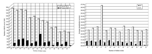
Fig. 6. Number of MLPs (out of 1000) with classification success greater than 89% (left), and average classification success (right) for these MLPs. Results are for the images of Fig. 5.
