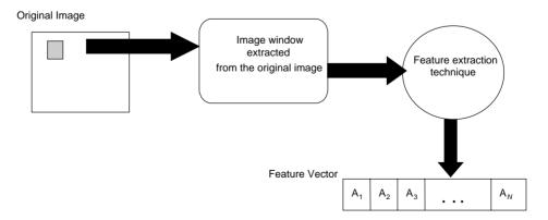
Fig. 3. Stages in feature extraction.
