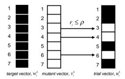
Fig. 4. Illustration of the crossover operation.
