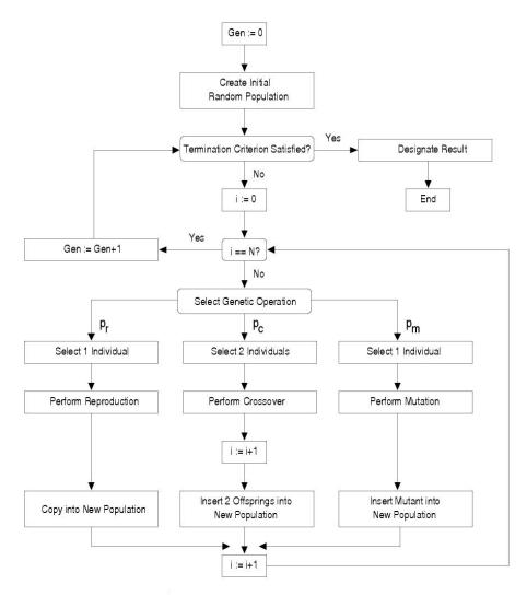
Figure 1: Flowchart of the operation of Genetic Programming
